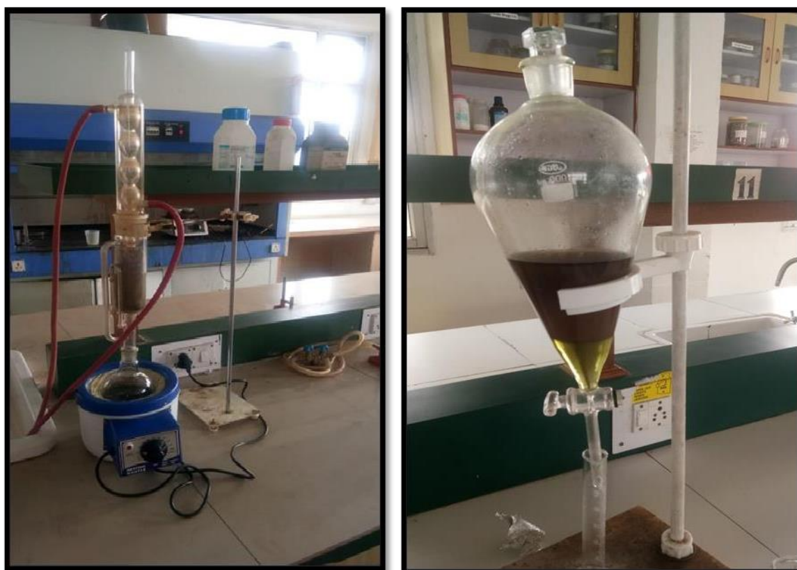
Figure 4 Extraction process in Soxhlet apparatus and fraction of plant material in separating funnel using a solvent
