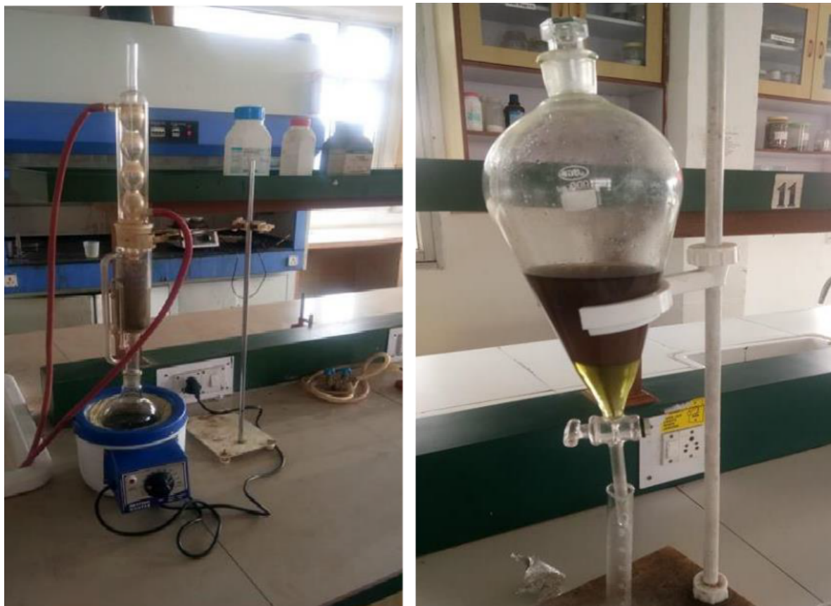
Figure 4. Extraction process in soxhlet apparatus and fraction of plant material in separating funnel using a solvent.
