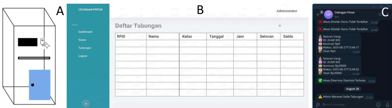
Figure 6. System implementation and user interface: (A) hardware prototype of the smart piggy bank, (B) website monitoring interface for real-time data visualization, and (C) Telegram notification output for automated saving transaction updates.
