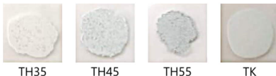
Figure 2. Homogeneity of hydroxyapatite-based toothpaste from freshwater mussel shells. Note: TH35 = 35% hydroxyapatite, TH45 = 45% hydroxyapatite, TH55 = 55% hydroxyapatite, TK = commercial toothpaste.
