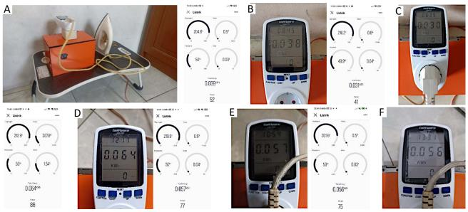
**Figure 1.** Comparison between system readings and reference measurements for the electric iron. (A) The electric iron used in the experiment, and (B–F) measurement results recorded at different time intervals.
