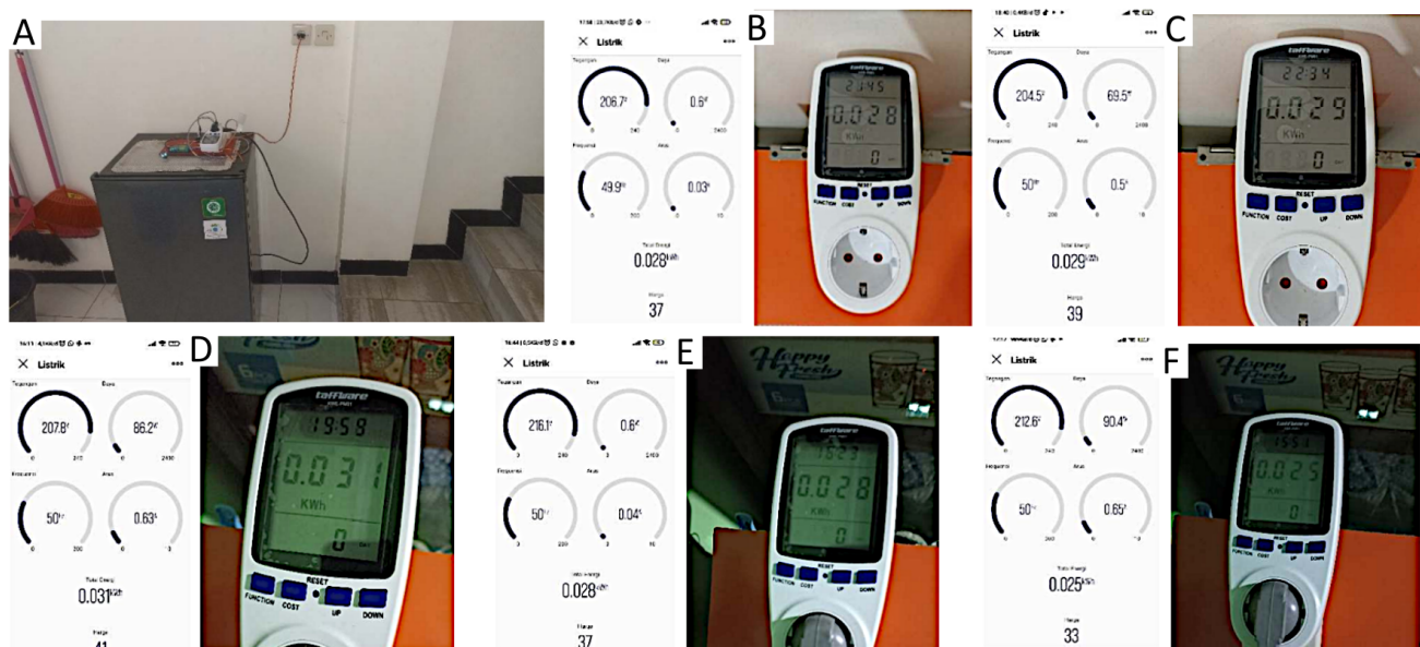
Figure 3. Comparison between system readings and reference measurements for the refrigerator. (A) The refrigerator used in the experiment, and (B-F) measurement results recorded at different time intervals.
