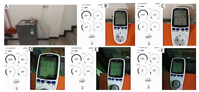
Figure 3. Comparison between system readings and reference measurements for the refrigerator. (A) The refrigerator used in the experiment, and (B-F) measurement results recorded at different time intervals.
