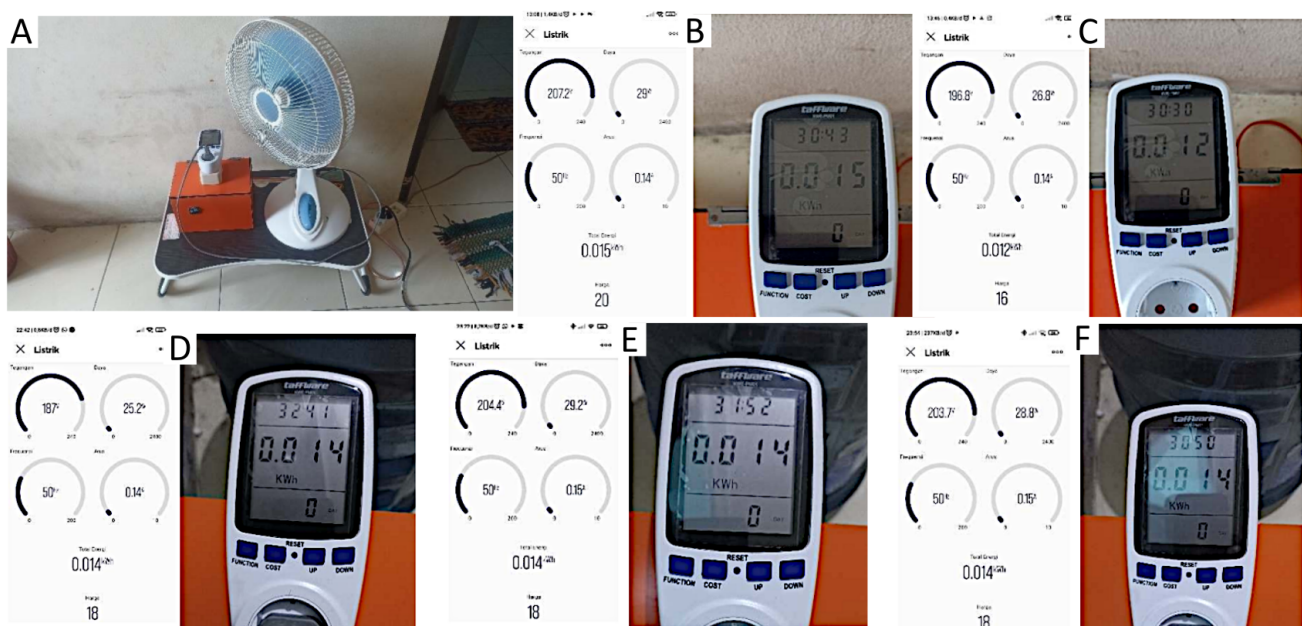
Figure 2. Comparison between system readings and reference measurements for the electric fan. (A) The electric fan used in the experiment, and (B-F) measurement results recorded at different time intervals.
